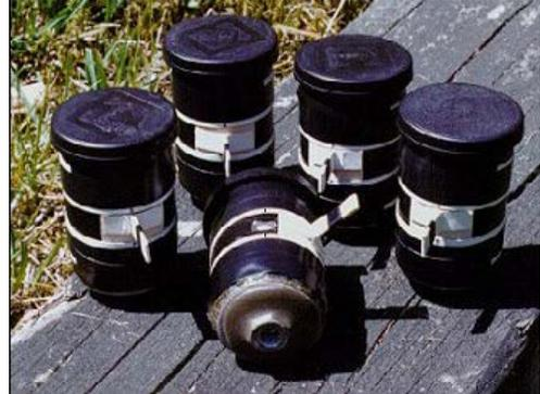
Figure 1. Pinhole camera made from a film canister
